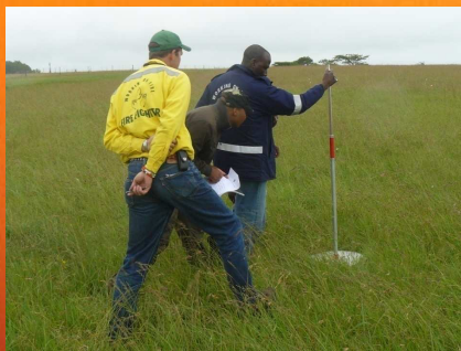
Measuring Fuel Load with a Disc Pasture Meter
